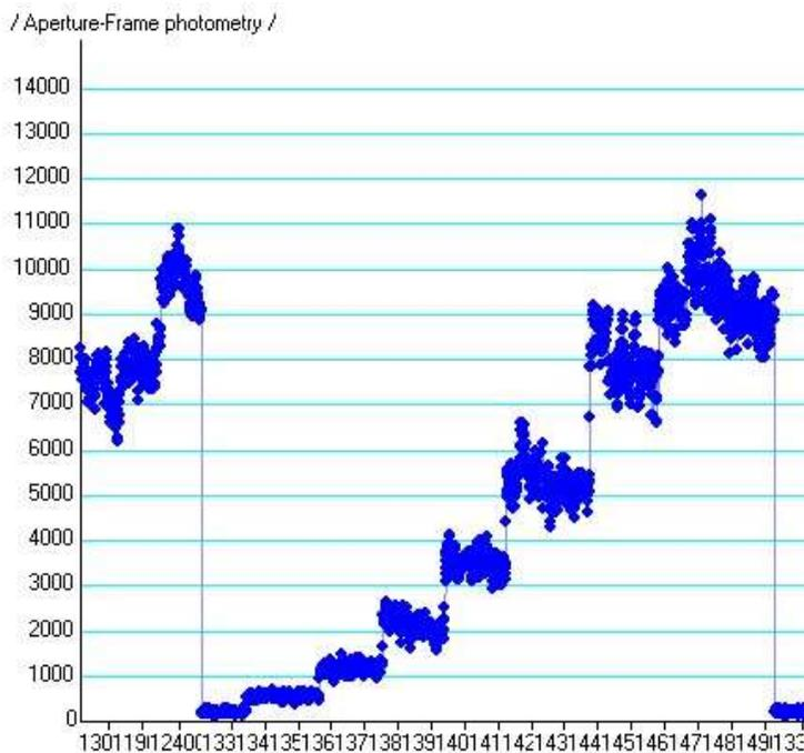
The increase in gain can be seen by the 9 steps visible in the light curve. One thing noticed in this light curve is that the gain setting at higher gain levels overshoots the initial gain and then stabilizes to a lower gain level. In practice, this should not be an issue for occultations, but for events where more
