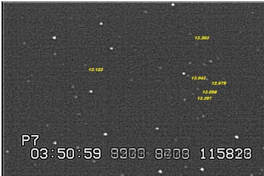
Stars down to magnitude 13.2 were visible. For occultations with large magnitude drops and 2-3 second durations, events with combined magnitudes of 12.5 could easily be captured with the Night Eagle on the 12-inch telescope at f3.3.
