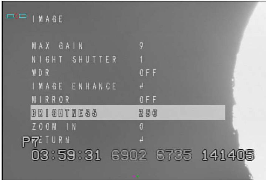
Brightness set to 8, notice that the glare is gone and lunar limb is visible. The brightness of stars approaching the lunar limb will be suppressed.
