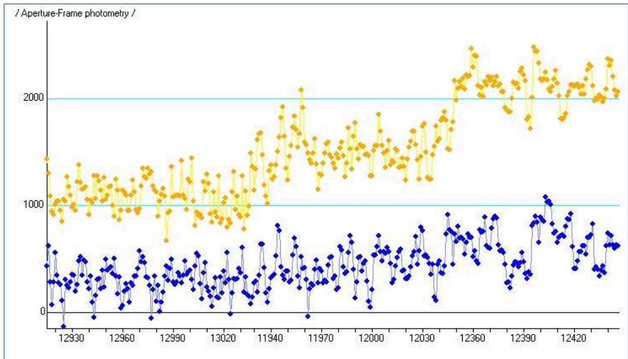
The gold trace shows three distinct steps in the star brightness between NS1, NS2, and NS3. Between NS1 and NS3, the measured brightness doubled. This allows the Night Eagle Astro to outperform other non-integrating CCD video cameras available for occultation astronomy.
