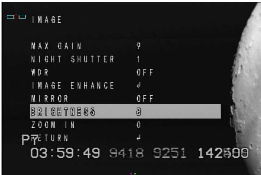
Observers of lunar occultations will have to find the best balance of Brightness setting to use for the brightness of the moon's limb and the brightness of the approaching star.
