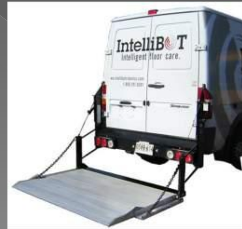
Tommy Gate lift 1000 pound lift capacity – greatly eases getting the scope in and out of a vehicle.
