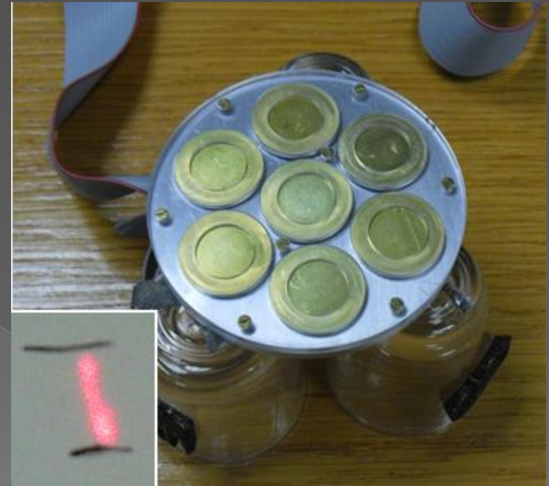
Prototype piezo transducer cell: elements deflect \pm 35 microns
