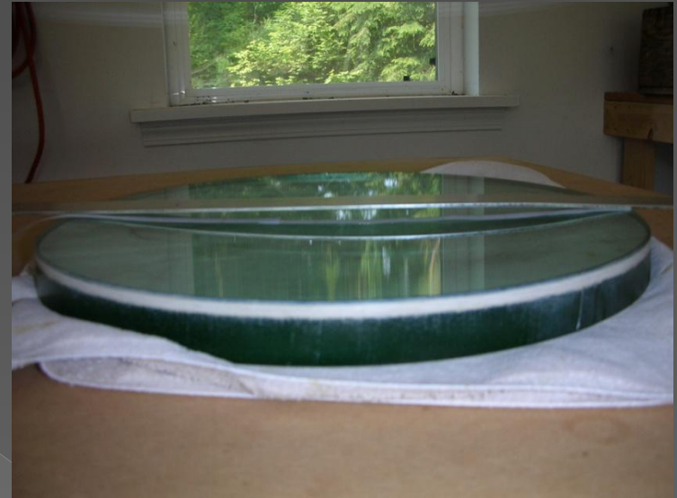
Mel Bartle's 13" soda lime slumped meniscus mirror
