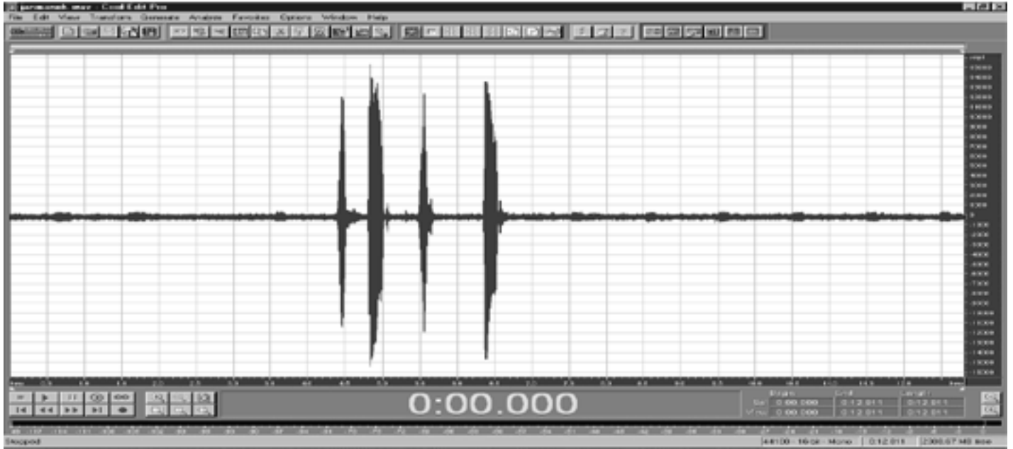
Figure 4. Example of recording by Harrie Rutten. This sample was recorded as 16-bit mono recording at 44100Hz sampling rate, resulting in a 1.1Mb large file for 12.8 second long recording. You can see weak, but regular, time marks of DCF signal together with Harrie's comments 'In' and 'Uit' two times.
